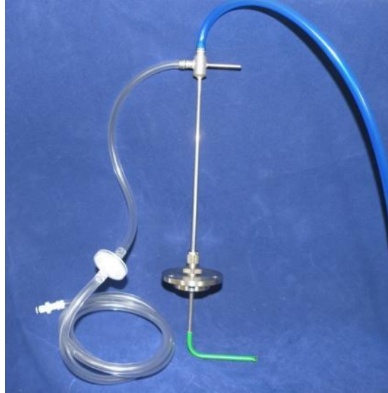
Figure 30—Example of a Pitot Tube
