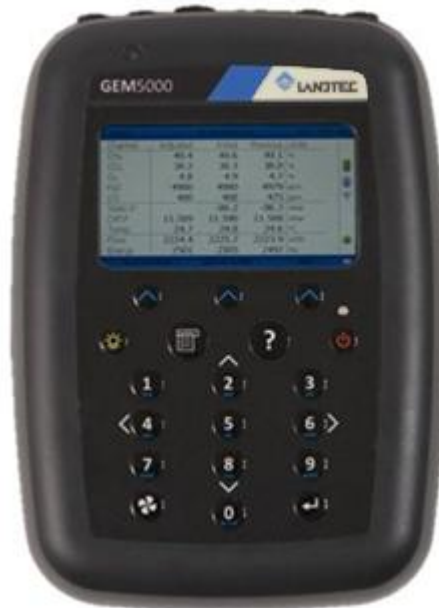
Figure 1—GEM5000 gas analyzer
